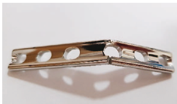
SLIKA 4. UZORAK PLOČICE PRIKAZAN ODOZGO NAKON CIKLIČKOG TESTIRANJA KOJE JE DOVELO DO LOMA FIGURE 4. A SAMPLE PLATE VIEWED FROM ABOVE AFTER DYNAMIC CYCLIC TESTING THAT LED TO BREAKAGE
