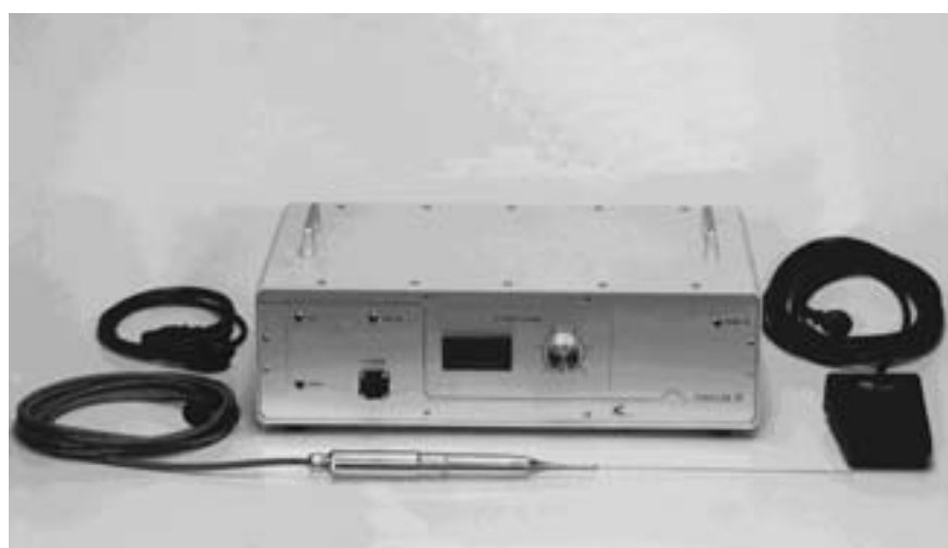
The neurosurgical endoscopic contact ultrasonic probe
