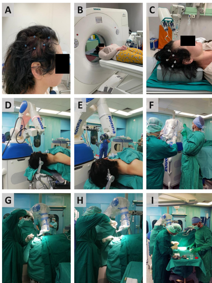
FIGURE 2. RONNA G4 surgical workflow. Before operation, the bone-attached screws are fixed to the patient's head under local anesthesia (A). The patient undergoes a contrast-enhanced preoperative computed tomography and magnetic resonance imaging according to a standard head protocol (B,C). In the preparation phase, the robot is positioned in an optimal position near the patient. An optical tracking system is used to coarsely position the robot with respect to the patient (D). The trajectory is visualized using a non-sterile probe (E). In the operation phase, after anesthesia induction, the operating field is prepared, and a sterile cover is put on the patient and the robot (F). Using the RONNAplan, the neurosurgeon selects the preoperatively planned trajectory following the tool guide positioning by the robot. Skin incision and burr hole drilling are performed manually by the neurosurgeon (G). A biopsy needle is advanced manually by the neurosurgeon to the target point in order to obtain the tissue for pathohistological analysis (H, I).
