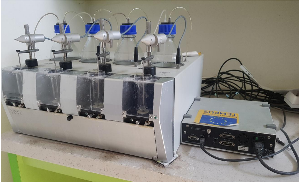
Figure 2. DMT-Tissue Organ Bath System-750TOBS used for in vitro force measurements of TSM (Danish Myo Technology, DK Aarhus N, Denmark)
