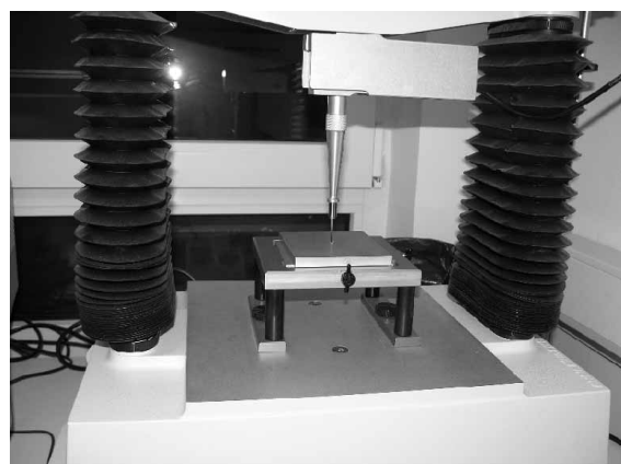
Fig. 3. Indentation testing of the rat femur.
