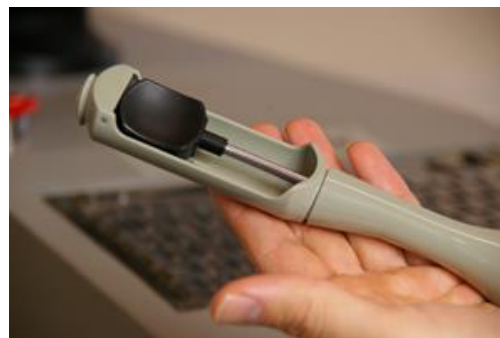
Figure 9. Transrectal probe for HIFU therapy. Courtesy of Sonacare Medical.
