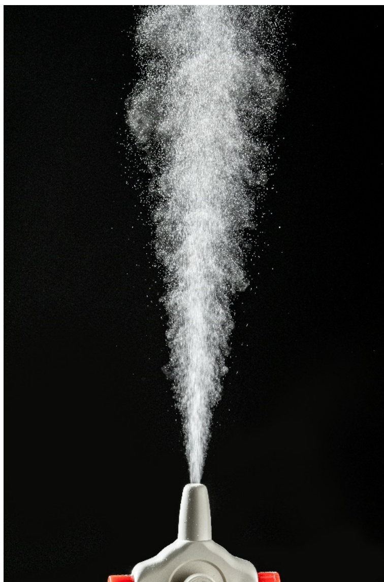
Figure 7. Spray cone of DSP-MS/Mannitol 1:9 upon aerosolisation with Miat ® insufflator.
