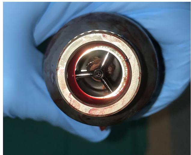
Figure 1 Thrombus inside the HM II LVAD.
