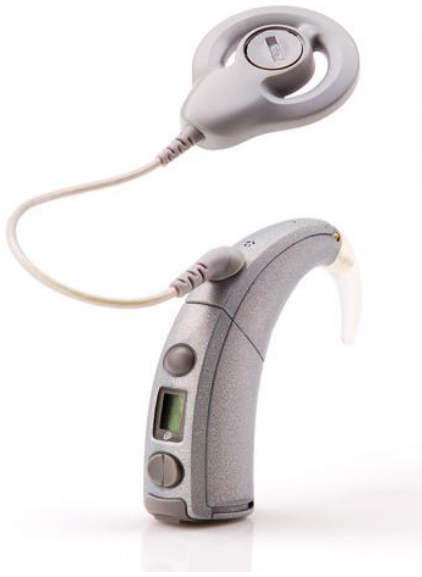
Slika 1. Zaušni procesor govora. Vidi se antena s magnetom. Photo provided courtesy of Cochlear™ Americas, © 2009 Cochlear Americas
