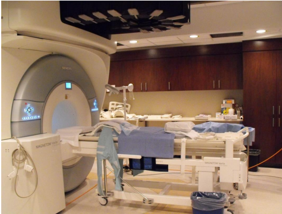
Figure 5. 3T-MRI scanner, interventional MRI tabletop with movable MRI table which can be undocked for patient transportation purposes.
