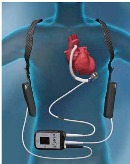
Slika 1. HeartMate 3 sustav potpore lijevoj klijetci (LVAD – od engl. left ventricular assist device ) Preuzeto iz: Thoratec Corporation HeartMate 3™ left ventricular assist system – Instructions for use.
