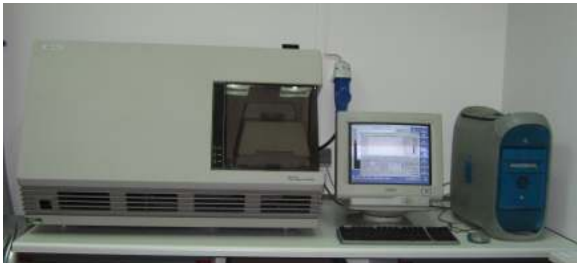
Slika 4.5 Instrumet ABI 7700 Sequence Detection System
