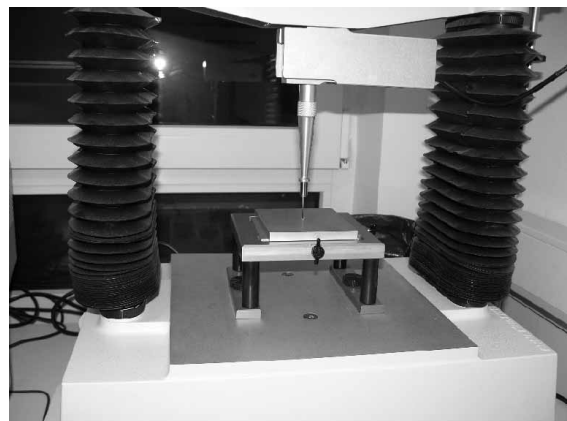
Fig. 3. Indentation testing of the rat femur.
