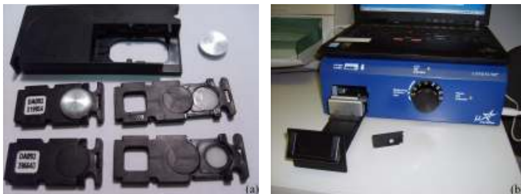
Figure 1. a) Landauer's OSL dot dosimeters with build-up caps and a plastic adapter for the reader, b) microStar reader.
