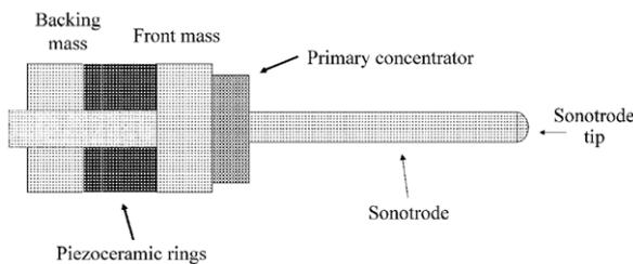
Fig. 1. Scheme of ultrasound probe used in measurements.
