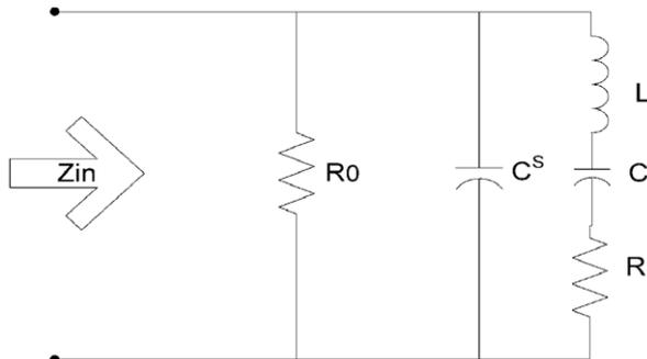
Fig. 4. Equivalent electrical circuit of the ultrasonic device.
