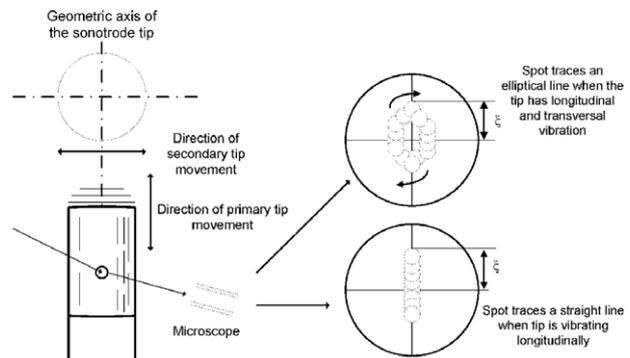
Fig. 2. Measuring the tip displacement using optical microscope.
